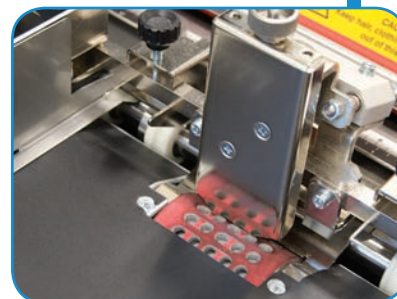
Rotating air-suction drum separates forms for accurate feeding
